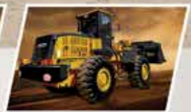
BL30-1 Front End Loader (Bucket 3.1 cum)
